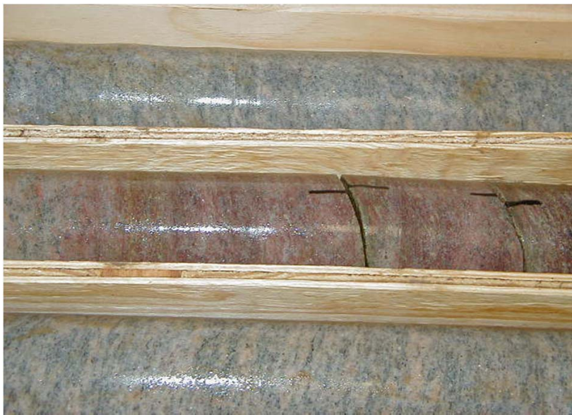
Reddish discoloration noted in R2
