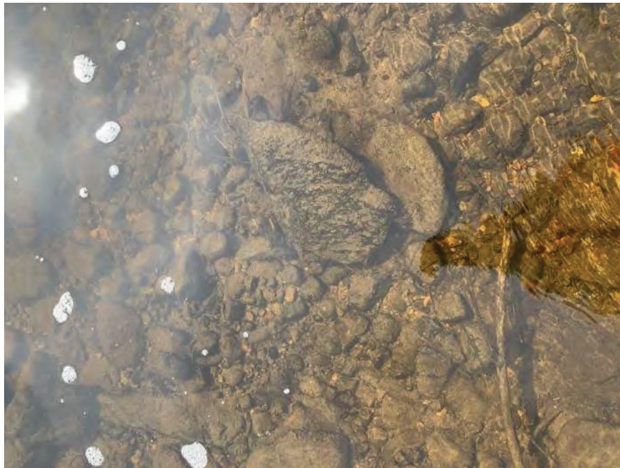
Photo 14: Streambed 5 ft from right bank 350 ft upstream of bridge. Streambed composition: 20% cobble, 60% gravel, 15% sand, 15% silt.
