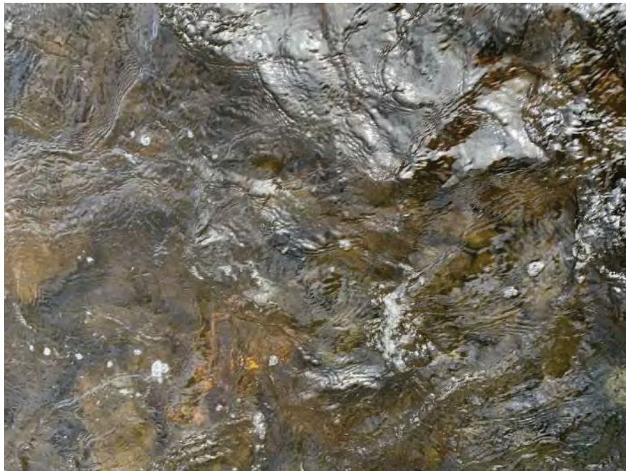
Photo 10: Streambed 5 ft from right bank 220 ft downstream of bridge. Streambed composition: 70% cobble, 10% gravel, 20% sand.
