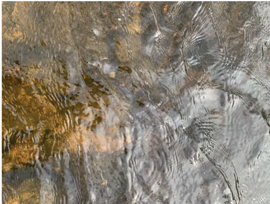
Photo 12: Streambed 5 ft from right bank 300 ft downstream of bridge. Streambed composition: 20% cobble, 50% gravel, 30% sand.
