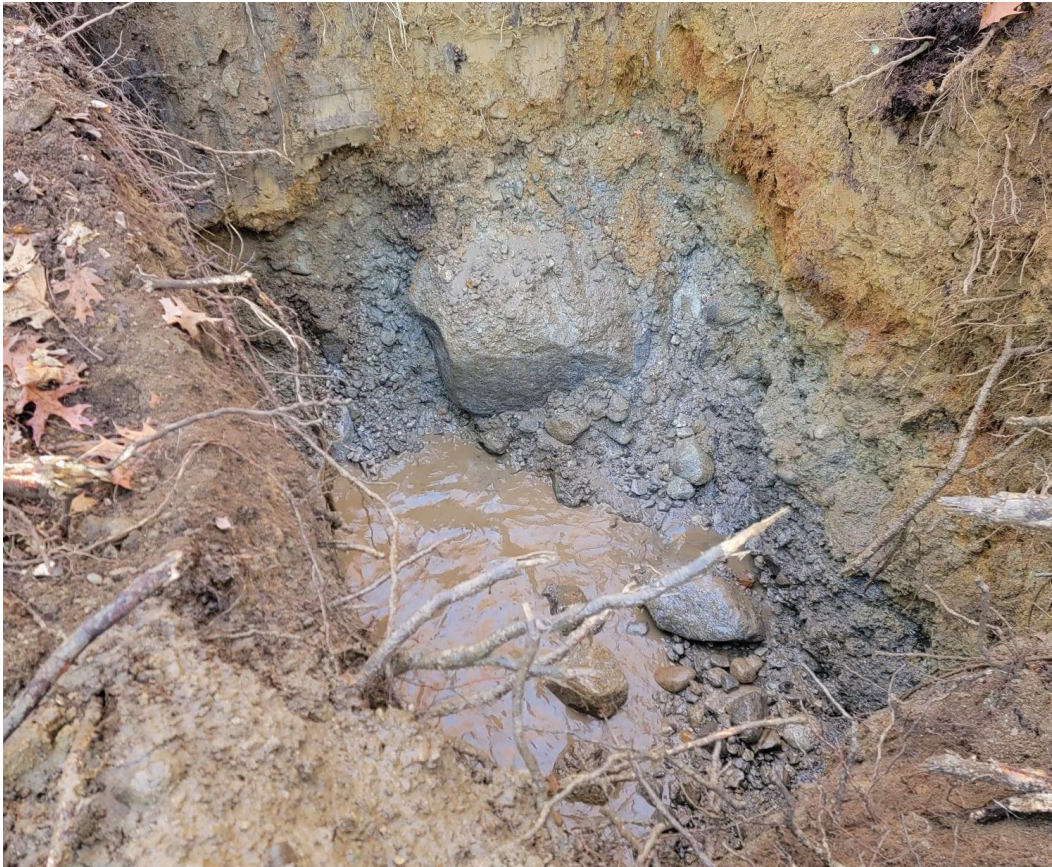
Photo 3: Bottom of GTP-3 with cobbles and boulders.
