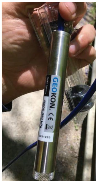
Photo 5 - View of vibrating wire piezometer before installation
