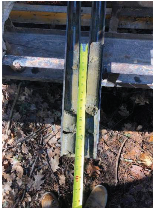
Photo 6 – View of glacial till in split spoon sample
