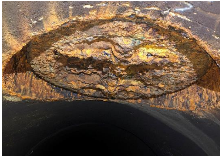
Manway 5: Boiler-Type, Corroded, No Cracks
