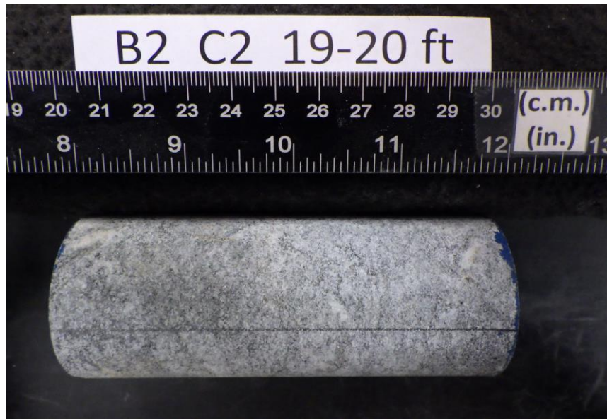
After cutting and grinding
