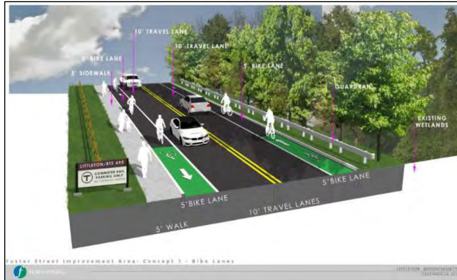
Figure 1: An Early Concept Alternative for Foster Street that was Not Selected Total Pavement Width is 35ft
