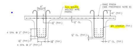
**Response #2:** Mild steel reinforcing bars may be used in place of welded wire reinforcement provided an equivalent area of steel is maintained and the bar spacing does not exceed 12".
