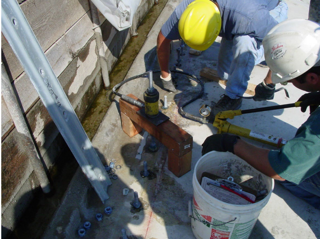
Pull Testing of clamp bar anchors
