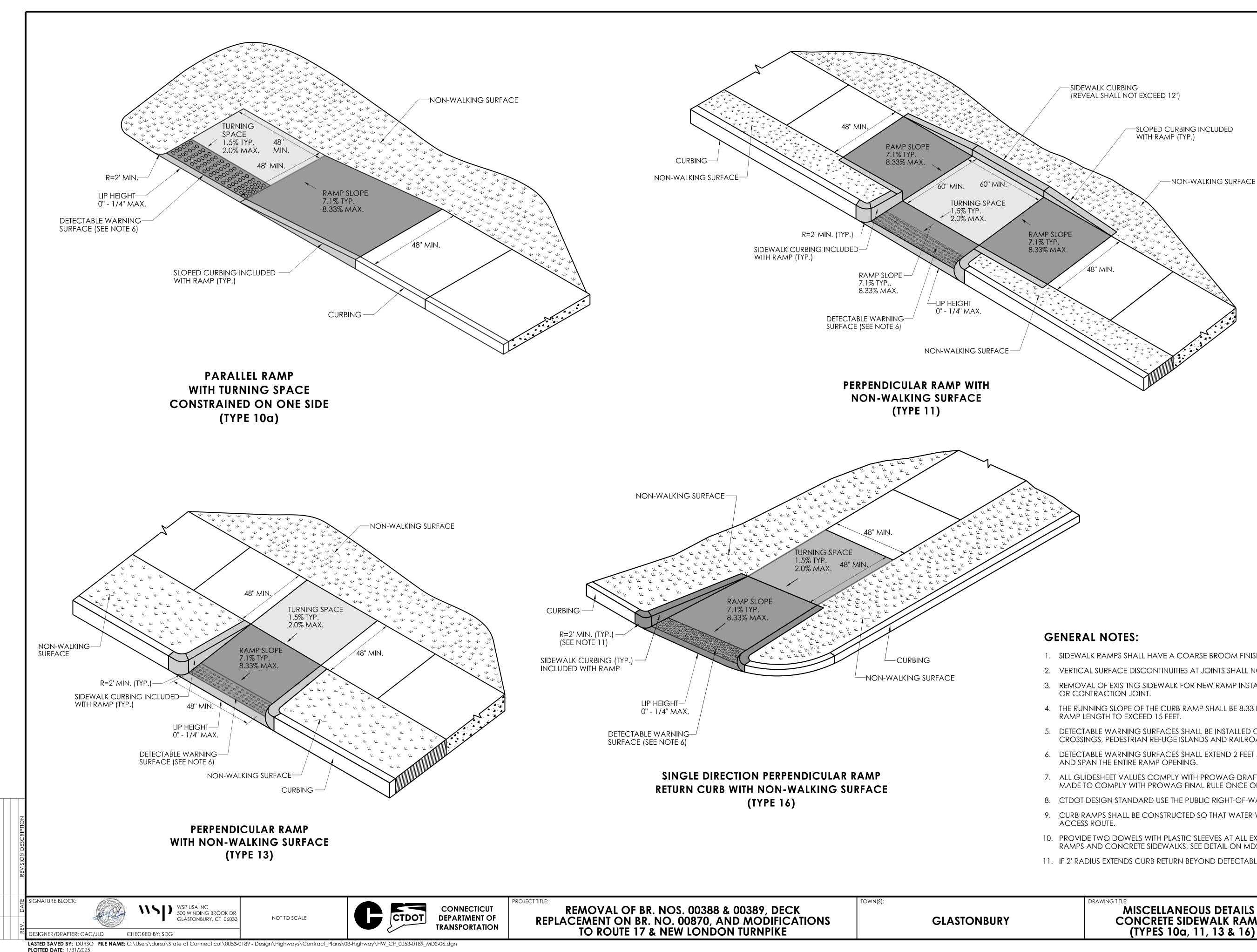
1. SIDEWALK RAMPS SHALL HAVE A COARSE BROOM FINISH TRANSVERSE TO THE SLOPE OF THE RAMP. 2. VERTICAL SURFACE DISCONTINUITIES AT JOINTS SHALL NOT EXCEED 1/4 INCH.
