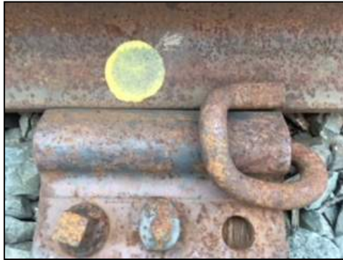
Correctly Driven Pandrol E-Clip as End of Clip Lines Up with Edge of Tie Plate
