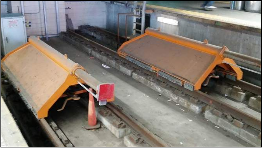
8b. High Energy Hydraulic Bumping Post
