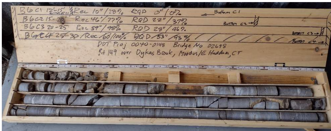
Boring B-6: Cores C-1 through C-4
