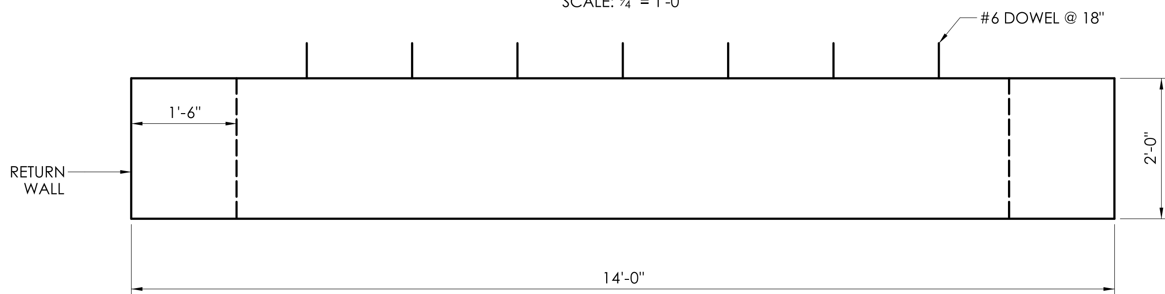
CUTOFF AND RETURN WALL ELEVATION
