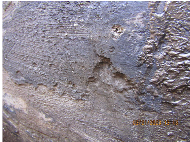
4 – Deepest Pitting in Pipe at Site 1
