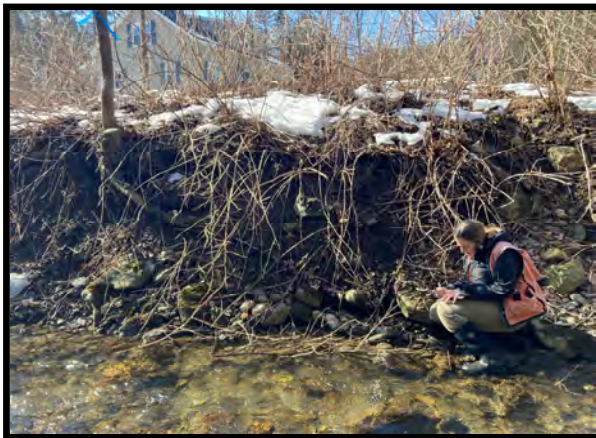
Photo 14: View facing the right descending stream bank at Bankfull Station 1+50, showing the stream downcutting and bank erosion. Photo taken February 15, 2023
