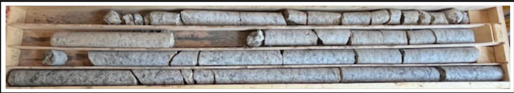
B1 & B2 BORING CORE BOX
